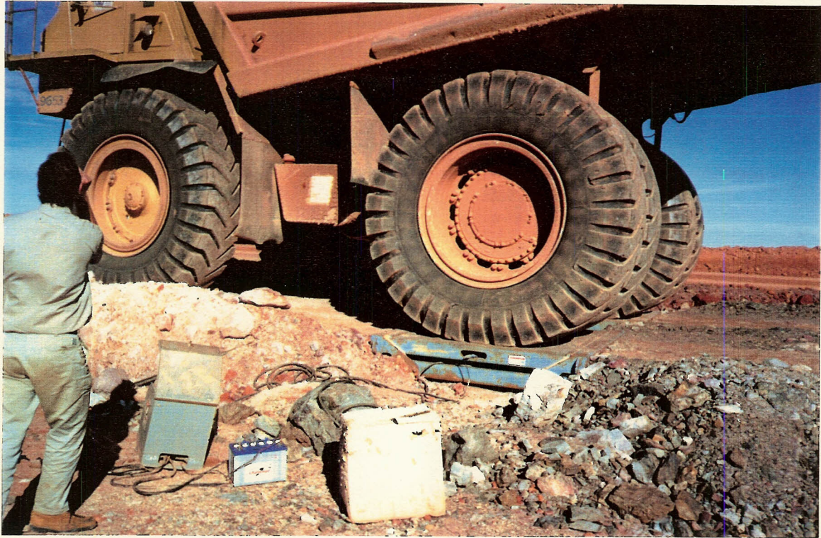
Photo 3. Test truck being weighed on platform scale.
