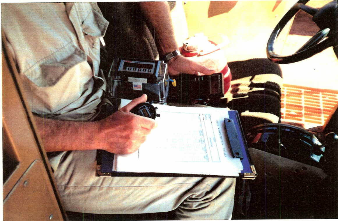
Photo 2. Data recording equipment set up in driver's cab. Minitrol volume recorder, digital thermometer, stop watch and data work sheets.
